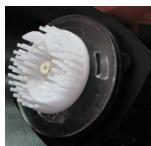
a bubble plate to reduce the turbulence in the reaction chamber;
